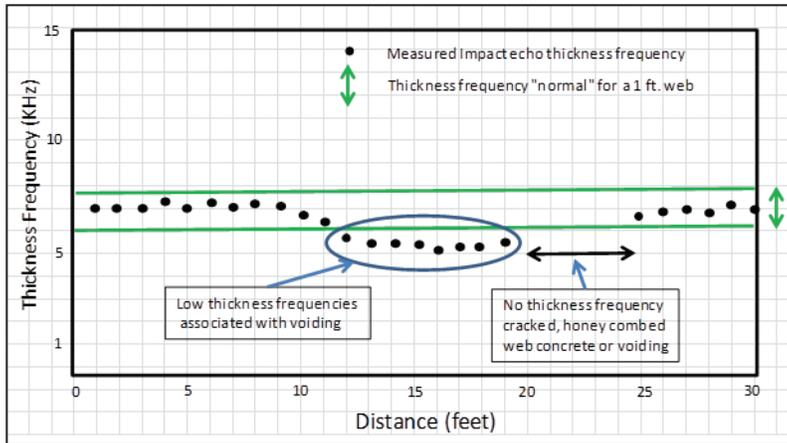
A plot of the recorded thickness frequencies determines suspect void/soft grout areas.
