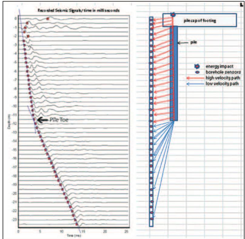
Diagram A: Parallel seismic measurements made in a borehole next to a timber pile to determine the length of the pile. These measurements use the timber pile as a waveguide and measure the time required for a wave generated on the pile cap to travel from the top of the pile to the end of the pile.
