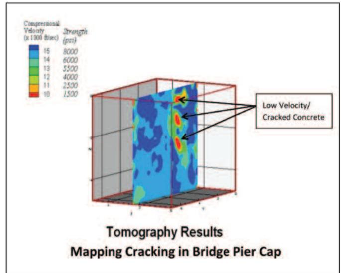
Diagram B: With access to two or more sides of a structure pulse velocity data can be acquired and evaluated with tomography imaging software. This software uses all the travel times acquired through a structure to make a best-fit velocity model of the data to produce a 2D velocity cross section or a 3D velocity image of the interior of the structure. This testing is very effective in identifying internal areas of weakened (cracked, voided, honey-combed, etc.) concrete.
